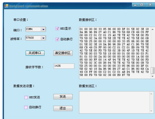
Figure 5.1: Data Receiving from Virtual Serial Port of MTS400CA
